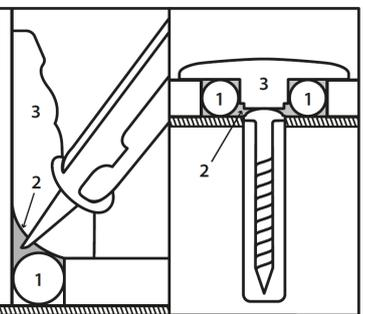
1. Tela PE / PE Foam Rod | 2. Silicone | 3. Molding / Rodapé
